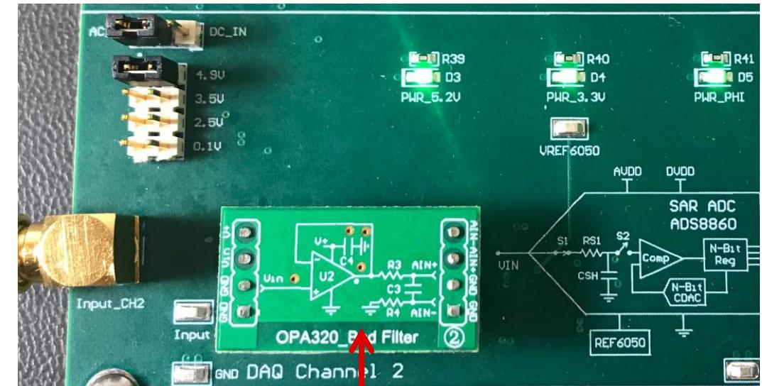
1. Install OPA320\_Bad Filter coupon card in socket.
