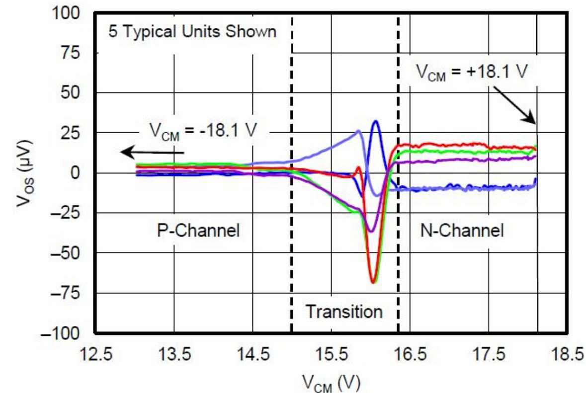
Figure 13: Offset Voltage vs. Common-Mode Voltage
