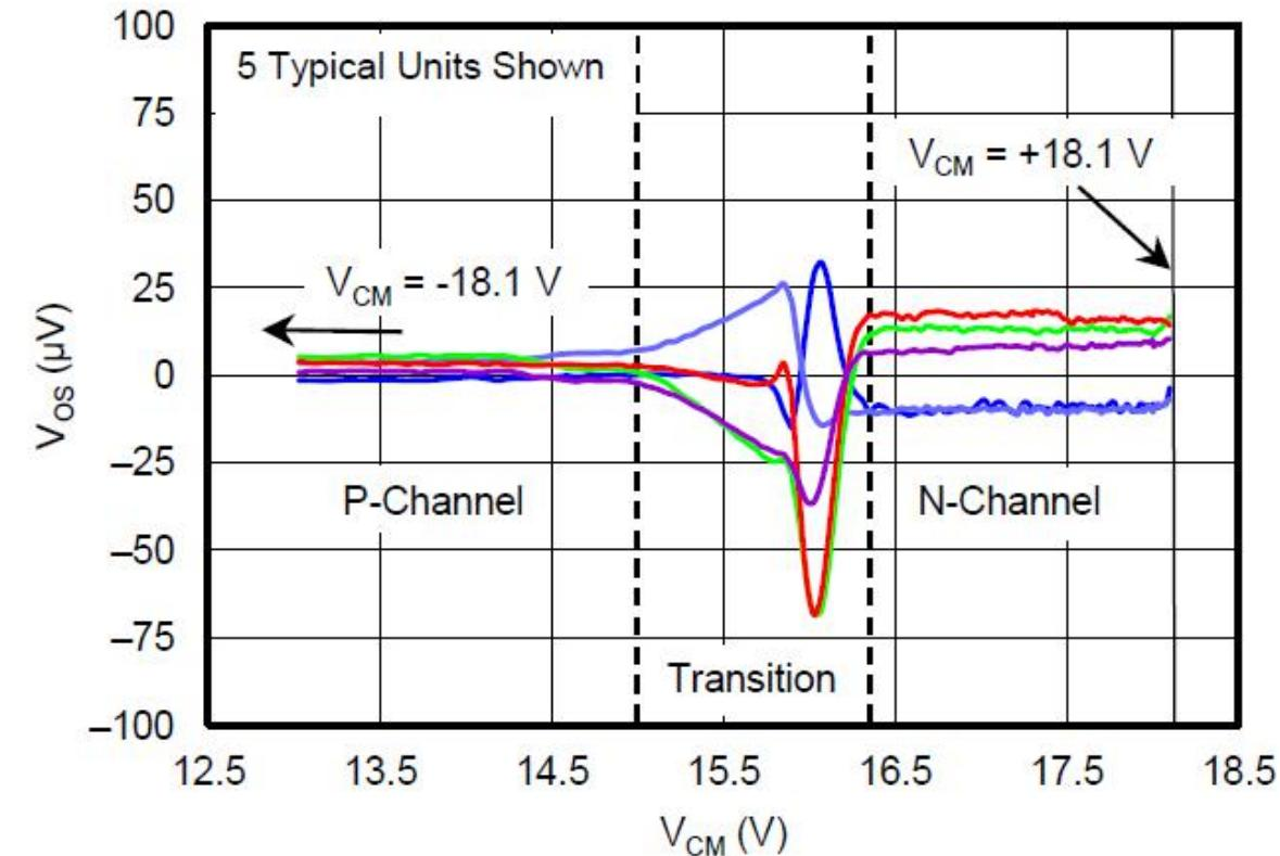
Figure 13: Offset Voltage vs. Common-Mode Voltage
