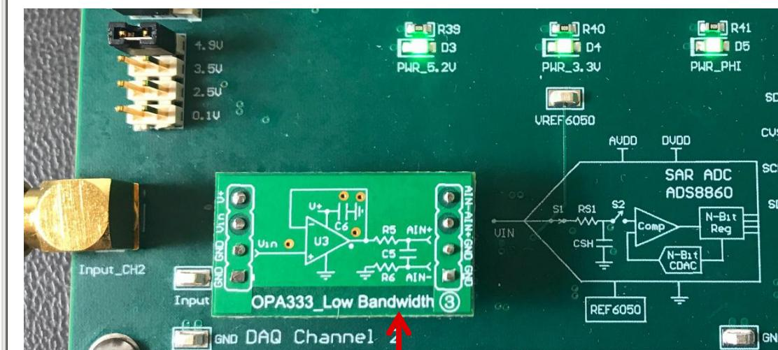
1. Install OPA333\_Low Bandwidth coupon card in socket.
