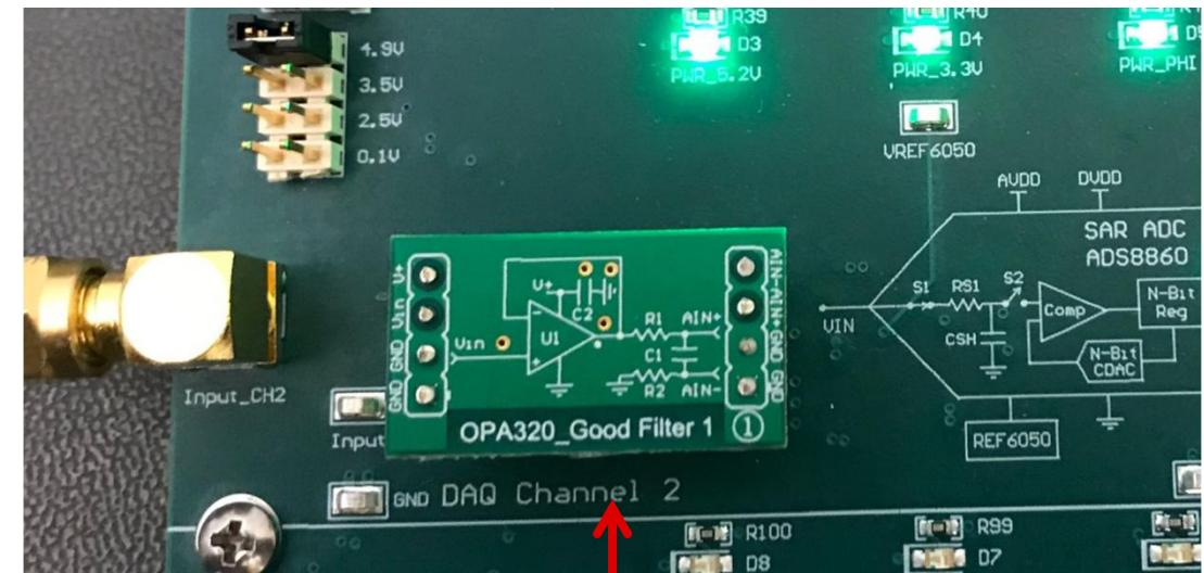
1. Install OPA320\_Good filter 1 coupon card in socket.
